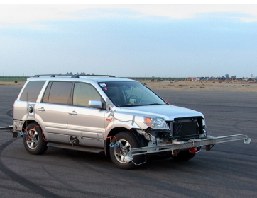
Full Scale SUV Rollover Resistance Test with AVC
