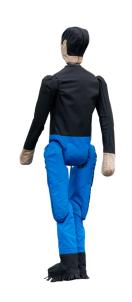
The Soft Pedestrian 360 is the next generation of articulated surrogate pedestrian target, bringing a whole new level of realism and vehicle protection to VRU testing.
